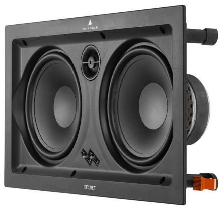
The SECRET LCR7 is a 2-way in-wall speaker equipped with two 170mm midrange/bass drivers with a polypropylene membrane, and a 25mm adjustable silk dome tweeter.
